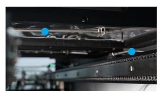
**Temperature monitoring**: Monitor temperature changes in the oven in real time, alarm when over temperature.
