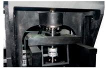
**Z-axis control** The lifting table improves movement rigidity through direct connection with the servo and ball screw. This enables precise control of the lifting position as well as controlled snapoff for improved printing yield.
