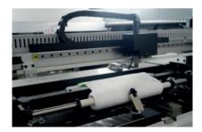
Dry/wet/vacuum cleaning module Three cleaning methods – dry wipe, wet wipe and vacuum wipe – make it possible to tailor your setup for a variety of cleaning needs. The precision spray system employs a top-down spray device that dynamically adjusts the spray amount and range based on PCB size, guaranteeing accurate cleaning results.
