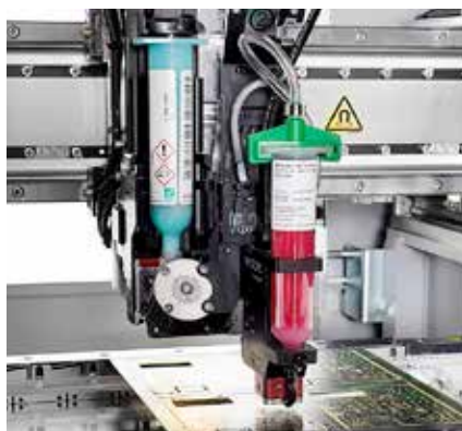
MY700 is used for high-speed dispensing of solder paste and adhesives.
