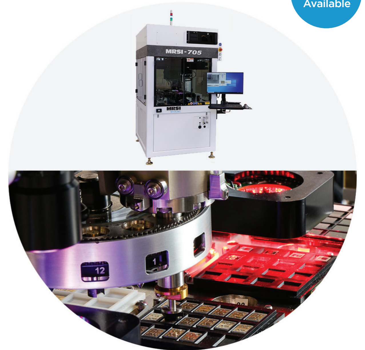
Patented turret for "on-the-fly" tool change
