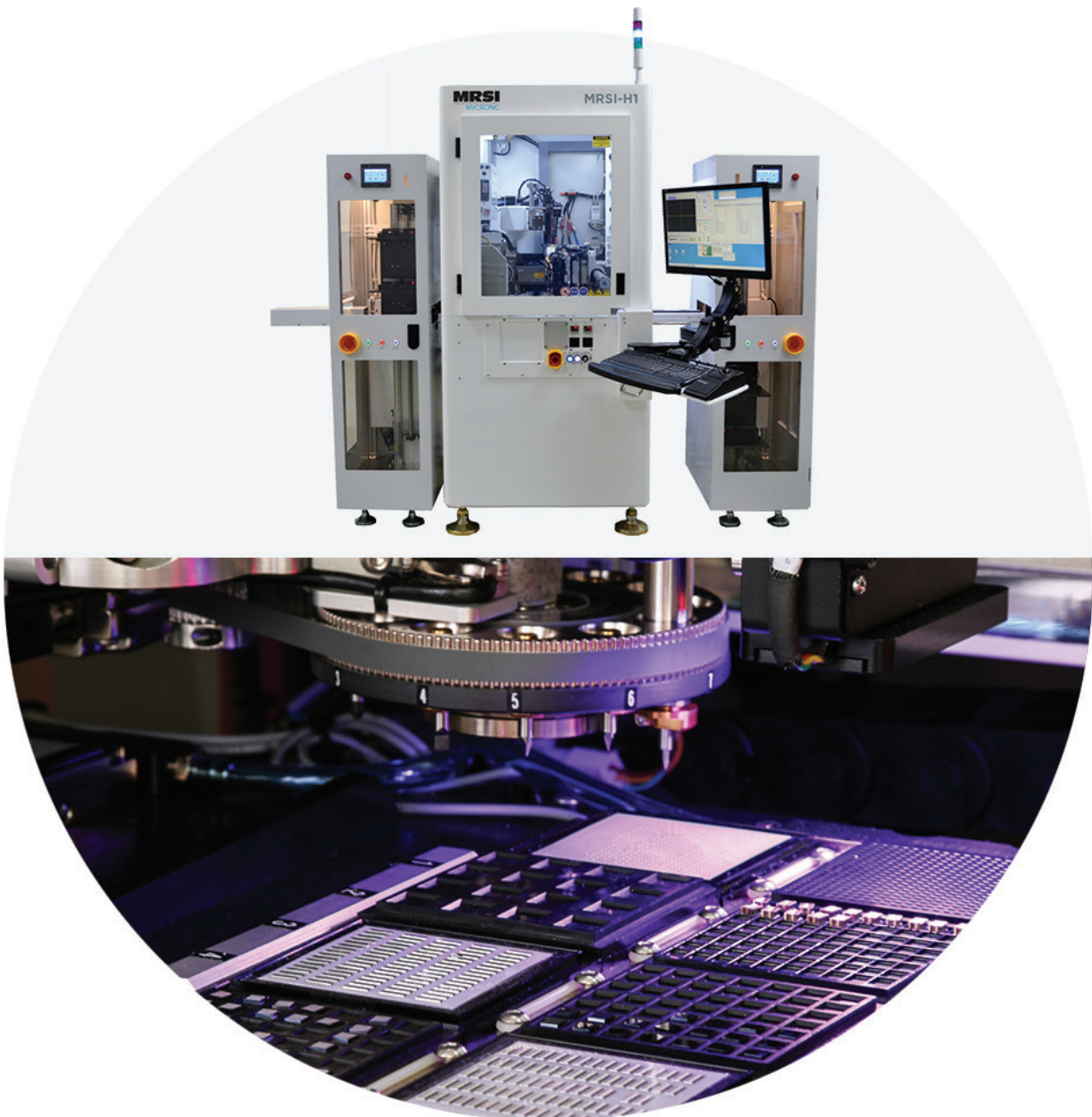
Patented turret for "on-the-fly" tool change
