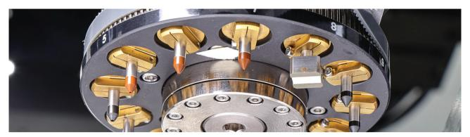
The MRSI-M3 offers an optional patented turret for "on-the-fly" tool change to significantly increase the production volume from our machine without sacrificing flexibility. The patented turret has the capacity for 12 tools with zero tool change time.
